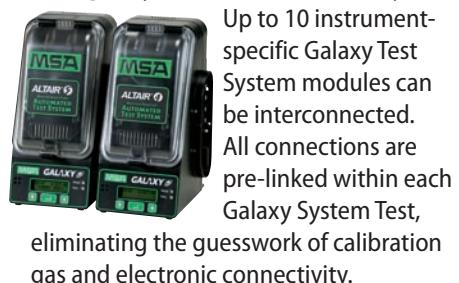
Up to 10 instrument-specific Galaxy Test System modules can be interconnected. All connections are pre-linked within each Galaxy System Test, eliminating the guesswork of calibration gas and electronic connectivity.
